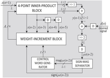
Fig. 1. Proposed DA-Based LMS Adaptive Filter
