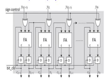
Fig. 3. Carry-Save Accumulator Block
