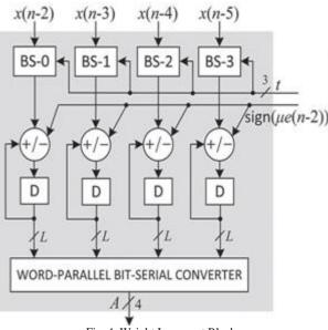
Fig. 4. Weight Increment Block
